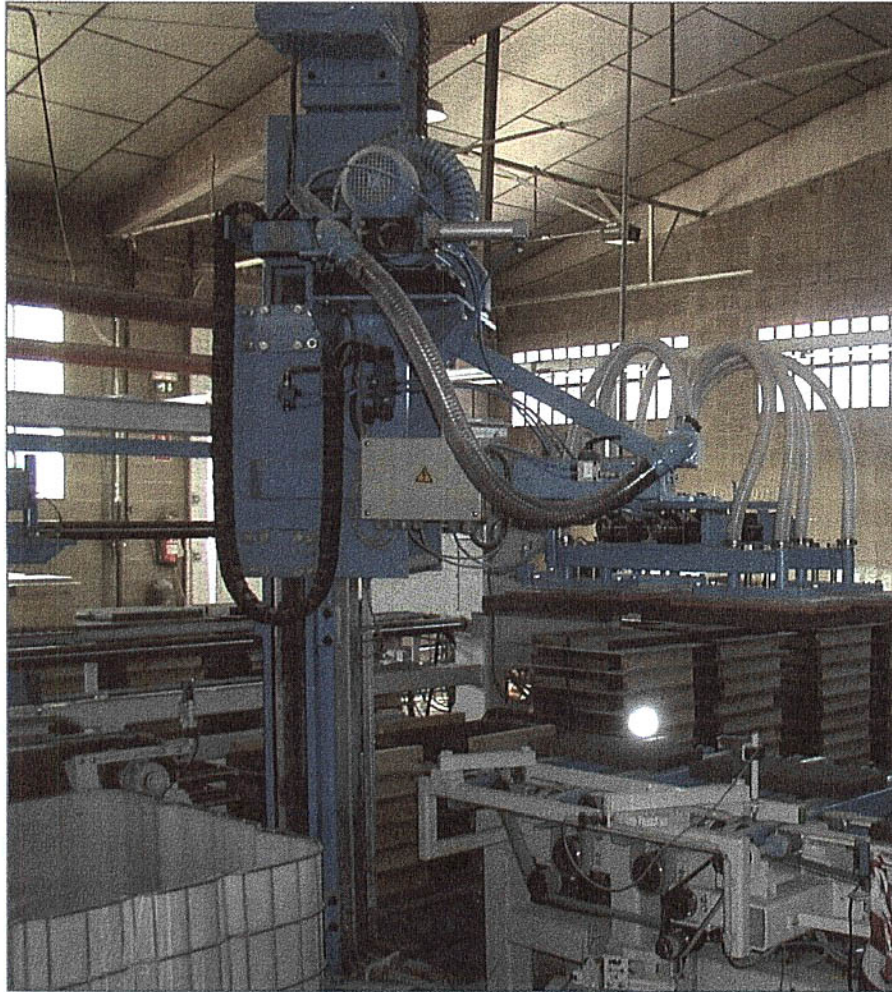
The high performance robot was developed for rapid transfer of the stones from the production machinery to the packaging machines.
